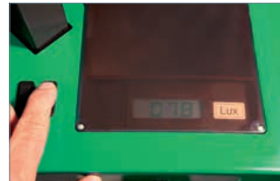
The digital luxometer precisely calculates the glare rating value of the low beam as well as the light intensity of the high beam.
