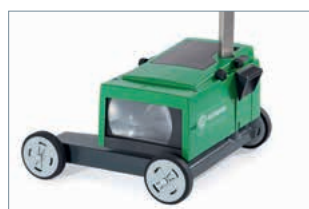
Optical housing can be lowered far down to test low sitting headlights.
