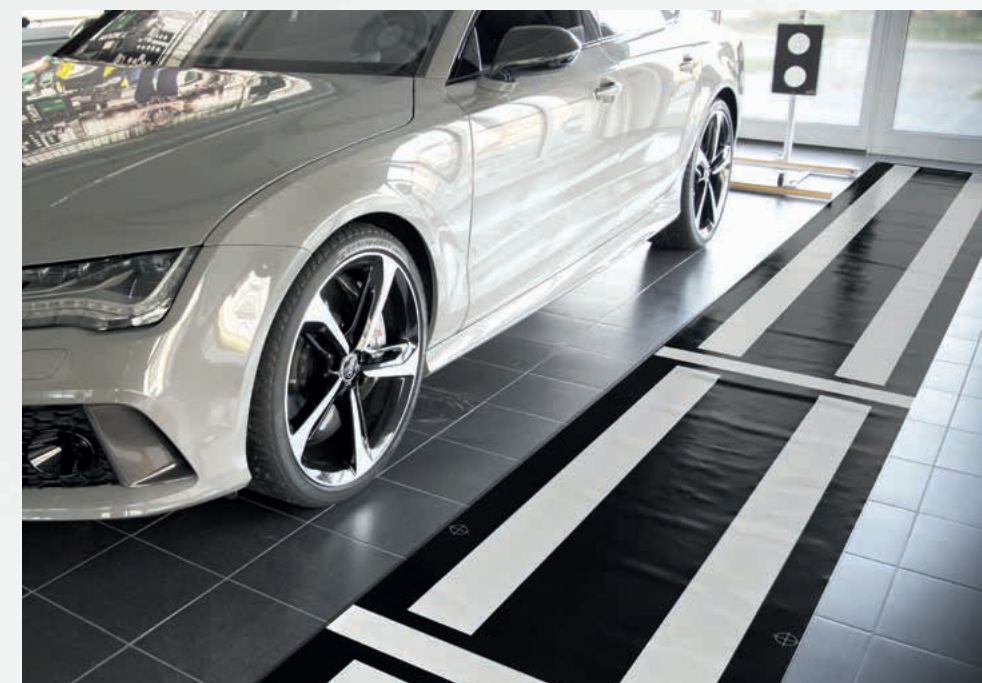
The additional kit Side for the exact calibration of the all-round vision camera system.
