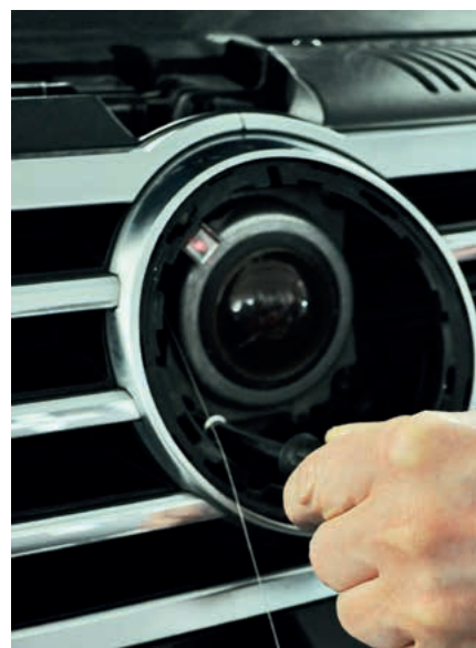
Reflection of the laser point on a radar sensor with mirror system.
