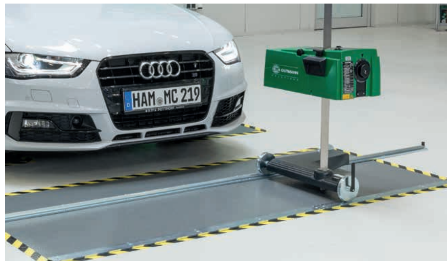
The adjustable rail system makes headlight measurement a doddle.
