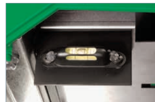
Spirit level for precise adjustment to vehicle ride height.
